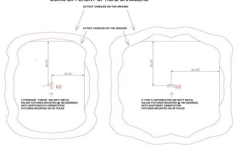
These fixtures are both produced by leading manufactures. The fact that the weaker performance comes from the less expensive manufacturer, while noted, is irrelevant. Both fixtures could originate from the same manufacturer and the results would still be evident. This is about understanding optical performance. The significant difference is the application of professional design and performance evaluation.
